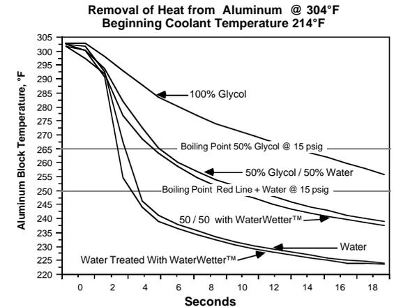
removal of heat from an aluminum bar at 304°F by quenching the bar in different coolants at 214°F under 15 psi pressure. Compare the time required to reduce the temperature of the aluminum to 250°F, or the boiling point of water at 15 psi. Red Line with WaterWetter® required 3.2 seconds, water alone 3.7 sec, 50/50 glycol in water required 10.2 sec, and 100% glycol required 21 sec. Water alone required 15% longer, 50/50 glycol 220% longer, and 100% glycol required 550% longer.
